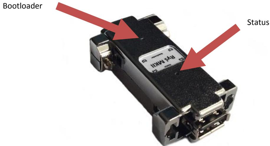
When pressing and holding the **Bootloader** button, one should connect the device via USB A-A cable to the PC running Windows. After being recognized by Windows OS, adapter switches into **Bootloader** mode which is confirmed with continuous pulsation of the **Status** LED.
